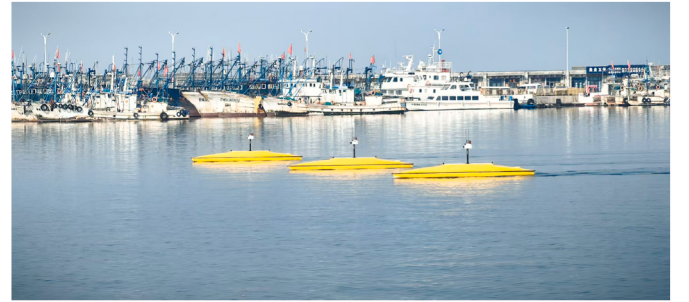
Fig. 15. Real-life photo of the line-formation figure-8 path-following test.
